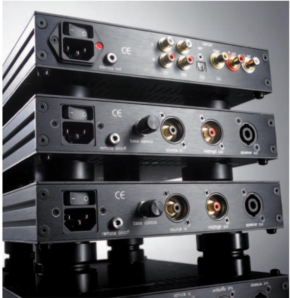
**Building a tower ahead of the dipoles: Daudio ideally likes to see its first product fired by its in-house electronics – a converter/pre-amp (top) sends a signal via RCA to two mono blocks. Via Neutrik Speakon socket it proceeds to the loudspeakers.**
